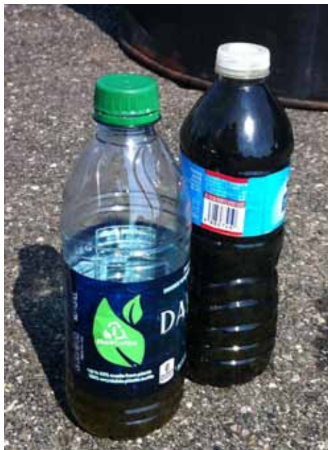
New brake fluid is not this colour (no, it's not ATE Blue)
