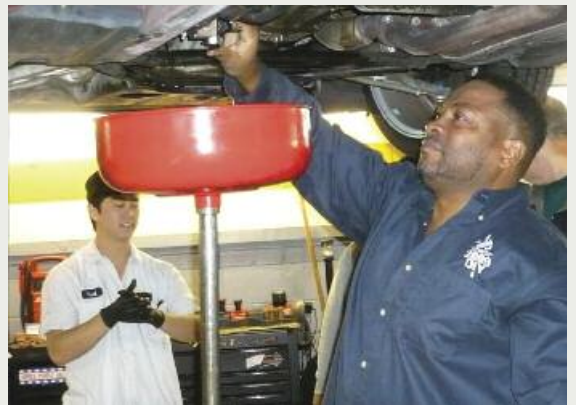
(Top right) Lothar Schuettler's 1964 3200 CS. (Center) Bill Warren draining the transmission fluid from his 1986 535i. (Right) Zachary Pullins replacing the fuel pressure regulator on his 2000 323i.
