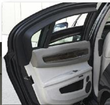
The BMW 7 Series High Security – Safety Glazing with Polycarbonate Layer
