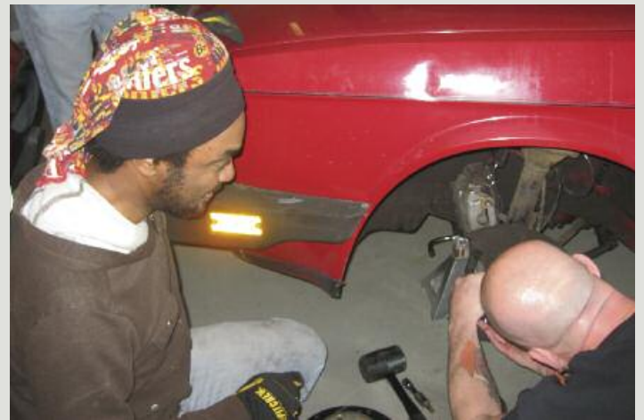
(Left) Daniel Hewes helping his Dad flush the brake fluid on their 1997 E36 318is. (Below) Bryon Sweeney and a Chapman technician replacing the front wheel hub on his 1986 E28 535i. (Below left) Denis Tharp replacing the clutch slave cylinder on his 1975 2002.
