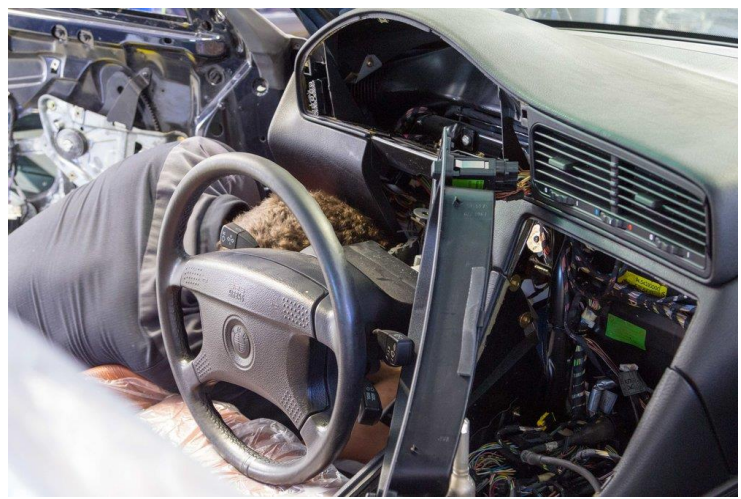
Swapping the pedal assembly from 2-pedal automatic to 3 pedal 6-speed by Coast Motorworks
